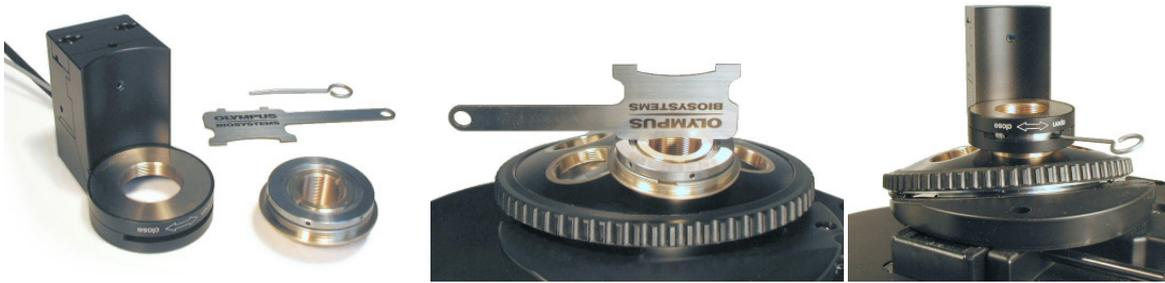
1. Disconnect the socket from the piezo-drive housing.
